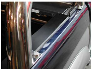
The front hoop of the roll bar is bolted in place using the rivnut previously fixed, and a ratchet strap may be needed to adjust the span of the two legs, to achieve required width. The rear roll bar fixing may use the rivnut method, or the nut and bolt method.
