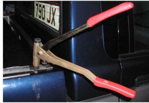
Remove the top cover and use a hacksaw to cut a notch out of the cover support bracket. The fitting of the rivnut is illustrated using a specialist tool, it can however be satisfactorily fitted using a small hand tool.
