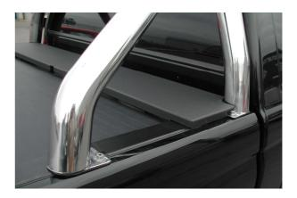
Cutting a notch from the corners of the roll and lock cover can be a simple square cut, or if you prefer, a circular hole may be neater, using a hole cutter or similar tool
